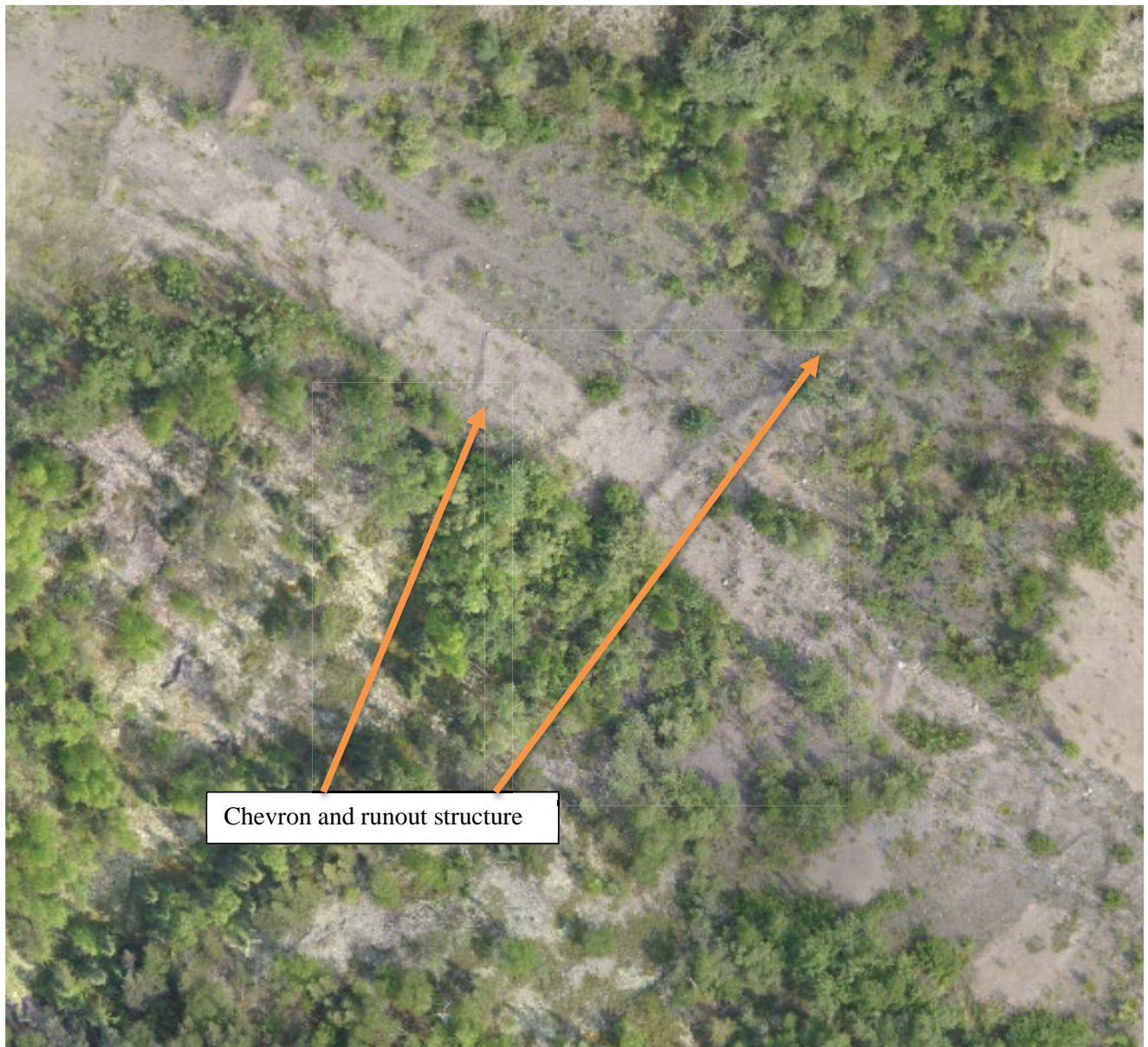
Figure 3. Fookes chevron and runout structure
