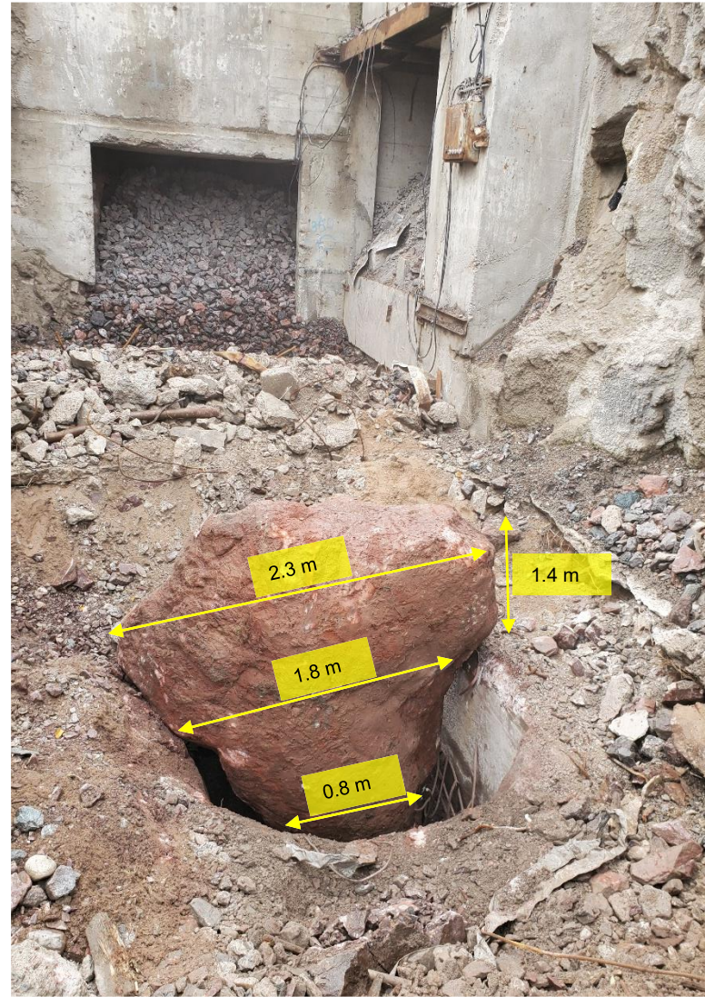
Photo 7: Dimensions of the pyramid-shaped boulder placed within Raise 3.
