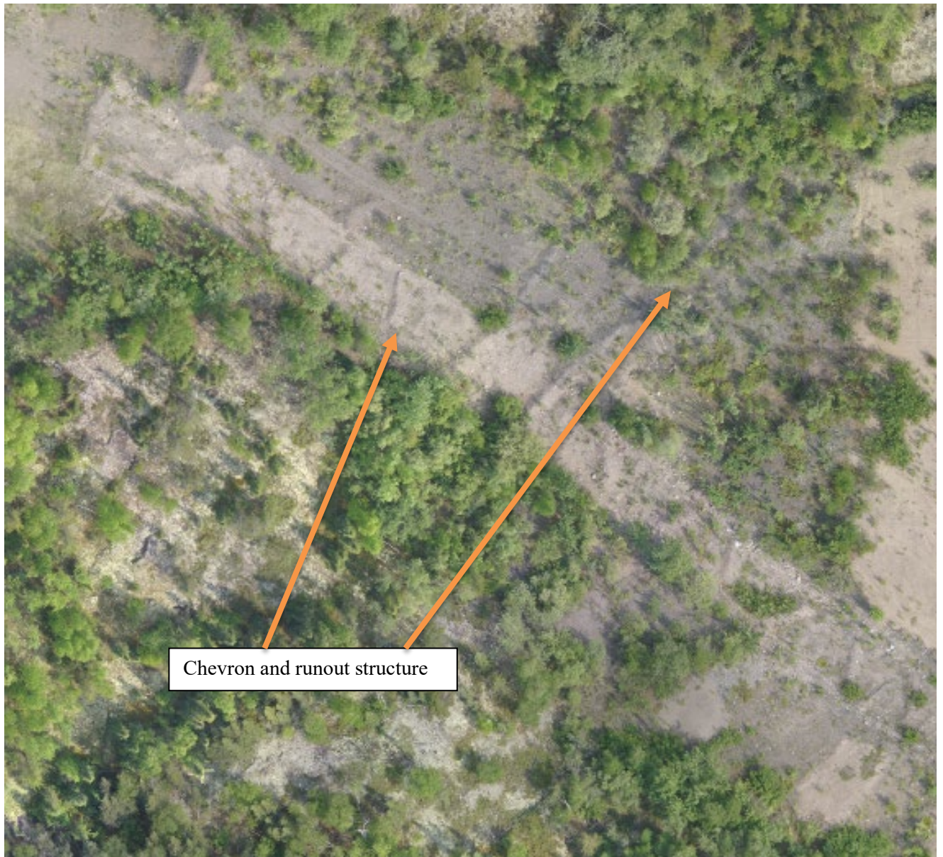
Figure 3. Fookes chevron and runout structure
