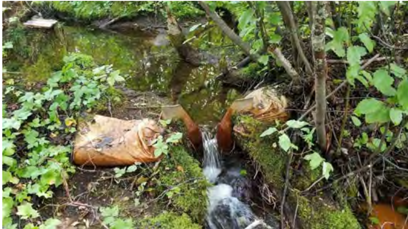
Photo 19 – V-notch weir used to estimate flow rate.
